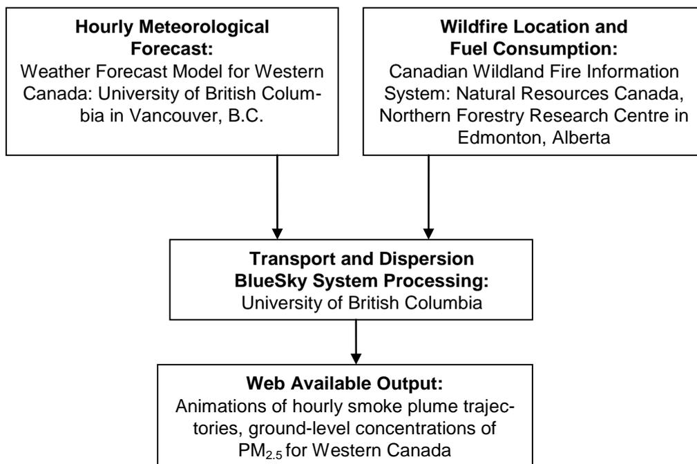
Figure 1. Structure and Components of the Western Canada BlueSky Smoke Forecasting System
